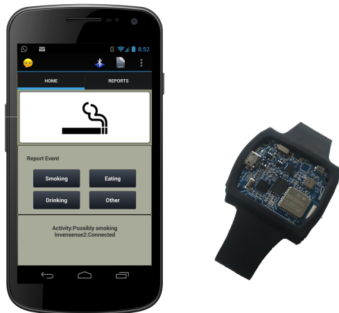
Figure 10: Smoking monitor mobile app and an IMU-equipped wristband.
